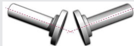
Angular Offset Misalignment
